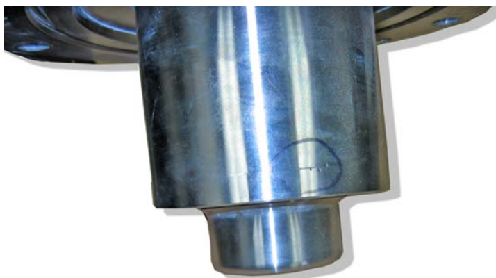
Rear casing breach caused by solids-laden vortices
