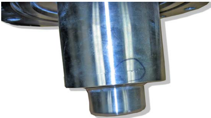
Rear casing breach caused by solids-laden vortices
