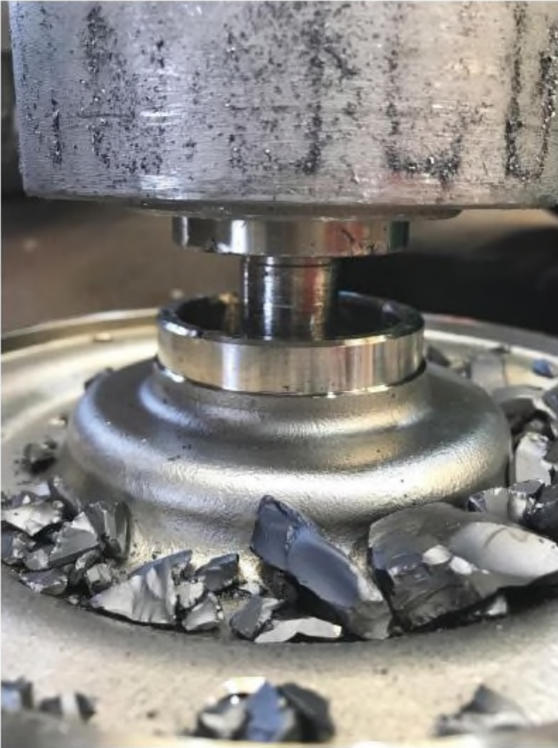
IMAGE 1: Broken silicon carbide bearing component (Image courtesy of Magnatex Pumps, Inc.)
